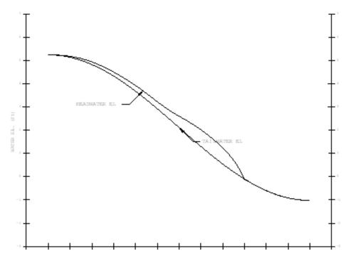
Headwater-Tailwater Relationships at Bridge (Note that the velocity of flow thorough the bridge is highest When the head differential across the bridge is greatest)
